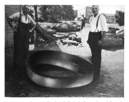
Here is a Disston band as it looked after a "wreck" at the J. W. Willis Lumber Company, Washington Court House, Ohio. It was 9-inches wide and was taken off the wheels by striking a piece of iron.
